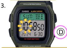
While the hour digits are flashing, press ① to change the number.
