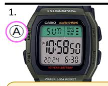
In the Timekeeping Mode, hold down (A) until the seconds start to flash.
